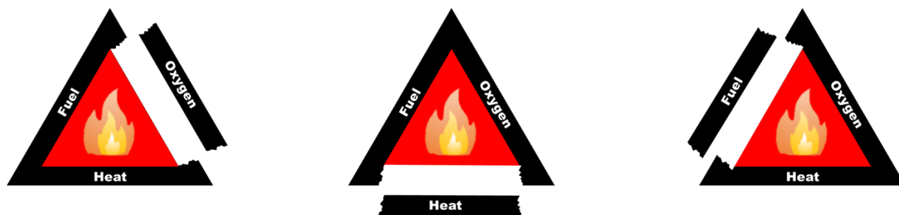
Figure 10. Removing and one of the three elements of the wildland fire triangle stops combustion
